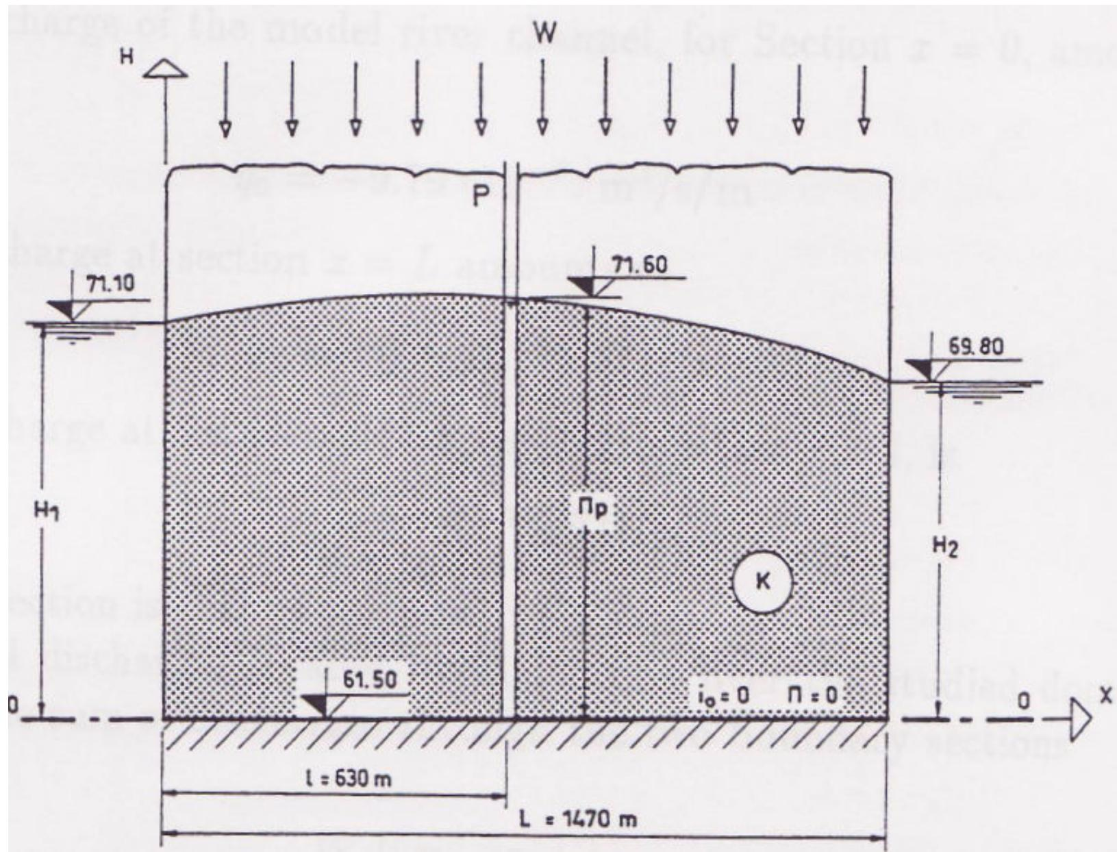
$$h = \sqrt{h_1^2 - \frac{(h_1^2 - h_2^2)x}{L} + \frac{w}{K}(L - x)x}$$
