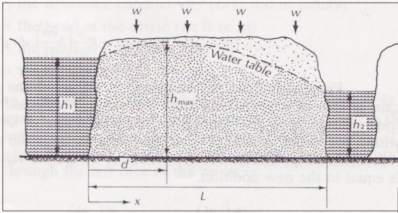
$$h = \sqrt{h_1^2 - \frac{(h_1^2 - h_2^2)x}{L} + \frac{w}{K}(L-x)x}$$
